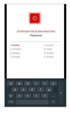
When a sensor is triggered, an alarm signal will be sent to the main and all synchronized monitors.
