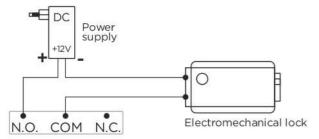
With such a connection in the power circuit of the lock, you must use the contacts: **COM** (switchable contact) and **N.O.** (normally open contact).
